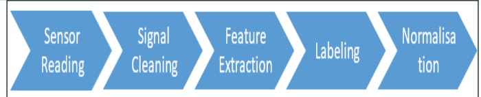
Figure 2: Data Pre-Processing Steps taken when Raw Data is Collected.
