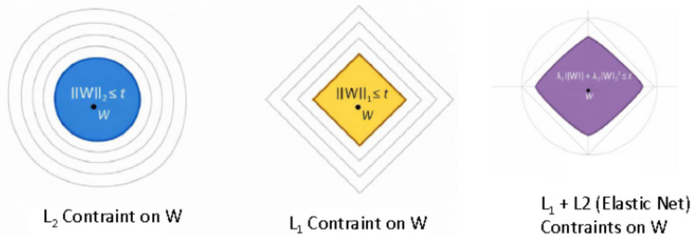
Figure 1: Level sets of L 2 , L 1 , and L 2 + L 1 (Elastic Net) regularization norms in parameter space. The L 2 norm produces isotropic circular geometry, the L 1 norm produces polyhedral sparsity-inducing geometry, and Elastic Net blends smooth shrinkage with softened sparsity structure.
